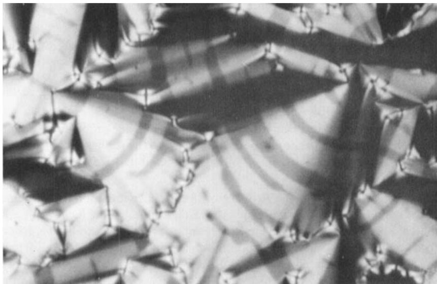
PLATE 8 Transition bars occurring at the A to crystal B transition for N -(4'- n -octyloxybenzylidene)-4- n -butylaniline (80.4) ( \times 100 ).
