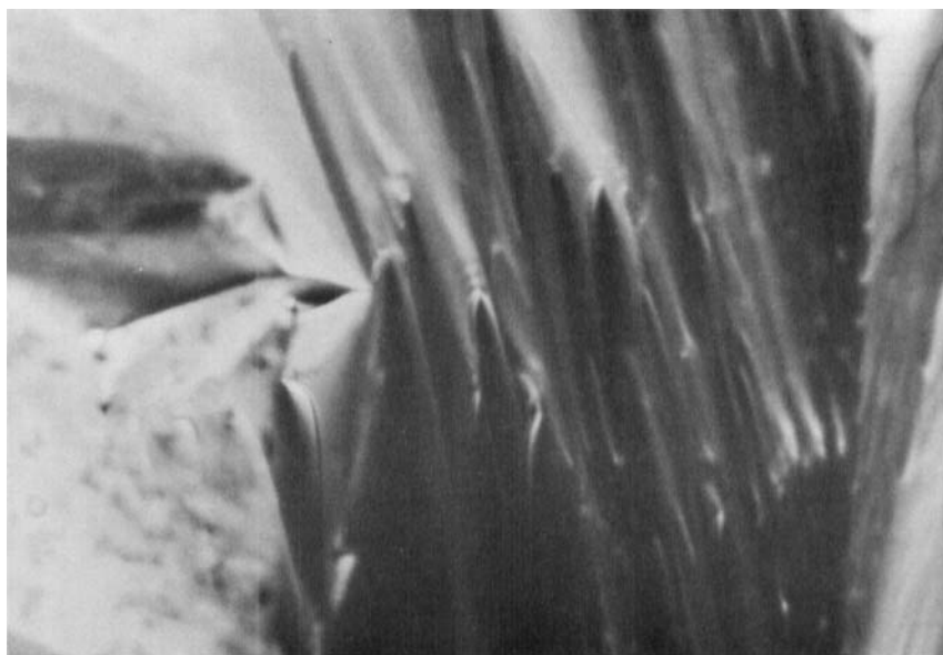
PLATE 6 The N-S_A transition 'barrier' as it crosses the contact region so destroying the parabolic focal-conic defects. The contact preparation is between N -(4'- n -butyloxybenzylidene)-4- n -octylaniline (left) and n -hexyl 4'- n -pentyloxybiphenyl-4-carboxylate (right) ( \times 100 ).
